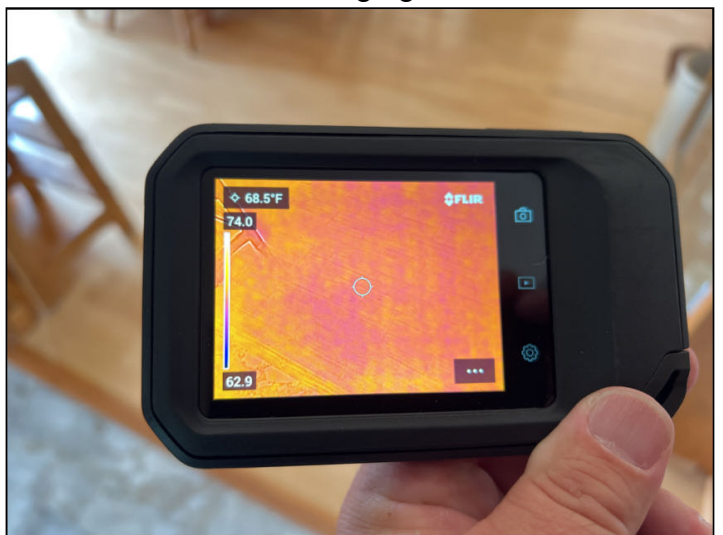
Radiant in-floor heating visible via thermal imaging
